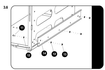
Secure the Support Bracket (Item 14) to the back of the Drop Down Table using M6 x 12 Button Head Bolts, M6 x 12 x 1SS Flat Washers and M6 Nyloc Nuts (Items 11, 12 & 13) using the holes shown.
