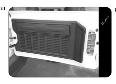
Remove the Cover Panel from the rear door interior panel by carefully unclipping it with a panel tool or similar.
