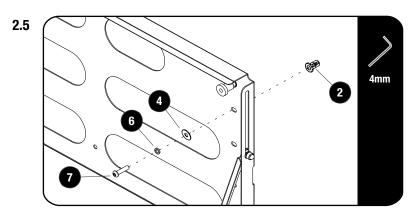
Secure the Drop Down Table using M6 x 25 Button Heads, M6 SS Spring Washers and M6 x 12 x 1 SS Flat Washers (Items 4, 6 & 7) as shown.
