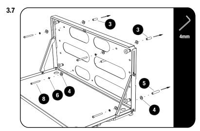
Insert two 30mm Spacers (Item 3) in the top two holes and two 35mm Spacers in the bottom holes drilled earleir in Step 3.5 and 3.6.
