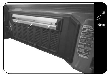
If your vehicle has the Sports Rail fitted, remove it by loosening and removing the 3 bolts shown.
