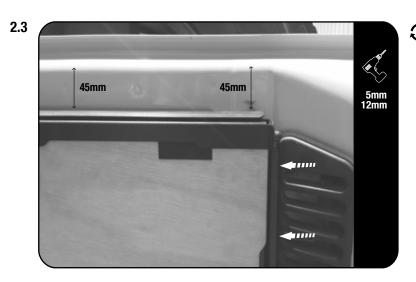
Drill 5mm pilot holes on the marks made in Step 2.2, using light pressure and taking care only to drill through the interior panel. Open the holes to 12mm.
