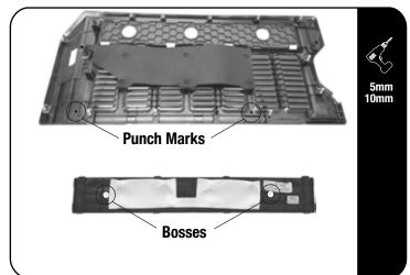
Looking at the inside of the Trim Panel, locate the two factory indicator marks shown.
