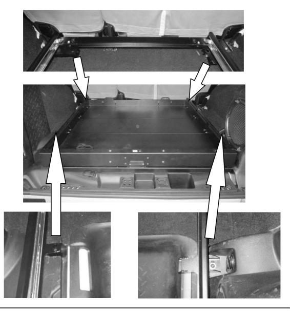
On certain models, it may be required to relieve the corners of the plastic recesses to allow the Cargo Slide's mounting feet to fit.
