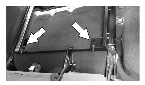
( **E** ) Open the Cargo Slide fully to expose the front mounting feet, as indicated by the arrows. Lift the front of the Cargo Slide and place the Front Mounting Strap (Items 2) underneath the mounting feet as shown.
