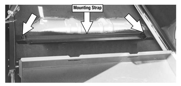
(F) Close the Cargo Slide and position it so as to sufficiently clear the rear door when closed. Once you are happy with the position of the Cargo Slide, carefully open the Slide as not to move its position and mark the location of the front mounting points (Refer to Step 3E) onto the vehicle's carpet.
