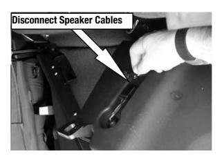
( **B** ) Remove the speaker box from the vehicle. Using masking tape, tape the area around the bottom left hand "mounting foot". Working on a suitable surface as not to scratch the speaker box, cutoff / remove the bottom left hand "mounting foot" as shown below. Refit speaker box to vehicle.
