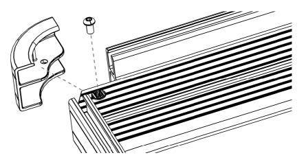
( **B** ) Loosely assembled a M8 x 25 Hex Bolt and M8 Nyloc Not to the two End Pieces and Joiner Piece (Items 1, 2, 3, 8).
