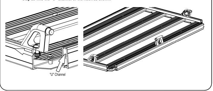
( **D** ) Starting on one of the Corners, loosen and remove the M8 Button Head Bolt securing the End Slat in position and slide / pull the Rear Slat backwards as shown.
