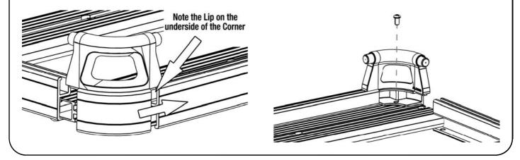
( G ) Assemble two Pipe A's (Item 1), one Joiner Piece and one Corner Piece together as shown below. Loosely secure the Corner Piece in position and slide the Rear Slat with assembled components back into position and secure the Rear Slat to the Rack using the M8 x 25 Button Head Bolts removed in Step 2D.
