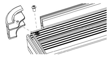
( **D** ) Loosen and remove the M8 Button Head Bolt securing either end of the Slat in position and slide / pull the Slat backwards as shown.
