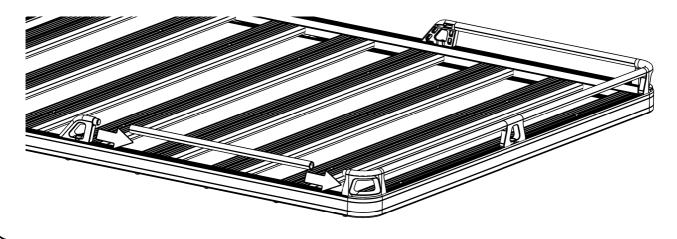
( H ) If either of the rear Pipes (Pipe A) are loose once your Expedition Rail has been assembled, you can loosen the appropriate section of Pipe and insert a C-clip Spacer (Item 9) over the taper of the Joiner or Corner as shown.
