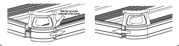
( **F** ) Referring Steps 2D & E, loosen and slide the open end of the Rear Slat out. Assemble the Steel Pipes (Item 5), Joiner Piece and remaining Corner Piece together as shown below and slide the Rear Slat with assembled components back into position. Secure the Rear Slat, Corner Piece and Joiner Piece in position.
