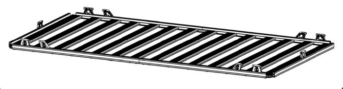
( C ) Assemble Pipe B and Pipe C to each "quarter" of the Rack as shown below and tighten all bolts. Should either of the rear pipe be loose, refer to Step 2L.
