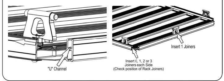
( **F** ) Slide a Corner Piece (Item 6) into the Slat making sure that the Lip on the underside of the Corner Piece slides into the Top Lip of the "U" Channel. Once the Corner Piece is all the way into the Rear Slat, loosely secure the Corner Piece to the Slat using one of the M6 x 12 Button Head Bolts (Item 4) supplied.
