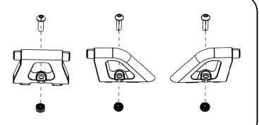
( C ) Referring to the images below, slide the two End Piece assemblies and the Joiner Piece assembly from Step 2B into the "u" channel of the Rack as shown.
