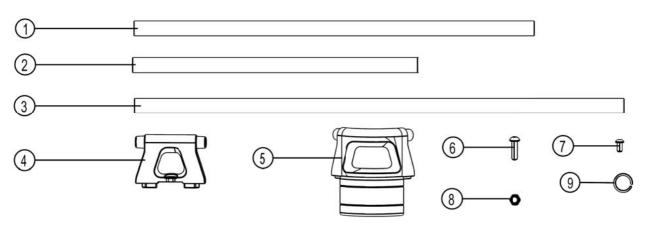
\* The lengths of Pipe A and Pipe B (Item 1 & 2) received in your Expedition Rail Kit will vary depending on the width and length of your Rack. Below are the various Rack widths and lengths of the two Pipes you should have received.
