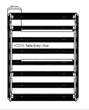
( D ) The Table Slides are slotted left to right to enable adjustment. Space the two Table Slides 550 mm apart and tighten all the Nyloc Nuts. Place a M8 Nut Cap (Item 6) over each Nyloc Nut.
