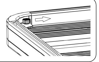
( **E** ) Place the Latch (Item 9) onto the Rack, lining up the mounting hole in the Latch with the Nyloc Nut inserted in Step 2D. Secure the Latch in position using the M8 x 20 Button Head Bolt and M8 Flat Washer (Items 7 & 8).
