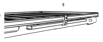
(**G**) Once the Rack has been mounted to the vehicle, open the Latch by pushing on the Latch Release and slide the Table into position. A small padlock can be used through the hole in the Latch Release should you wish to lock the table.
