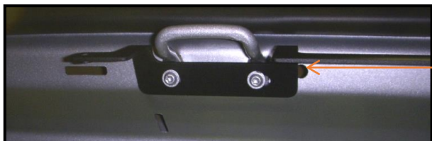
Keep this hole clear! It is used for the plastic windshield header alignment stud.
