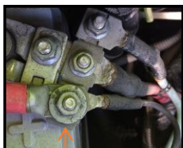
Positive side – 10mm socket
