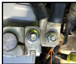
Negative side – 12mm socket
