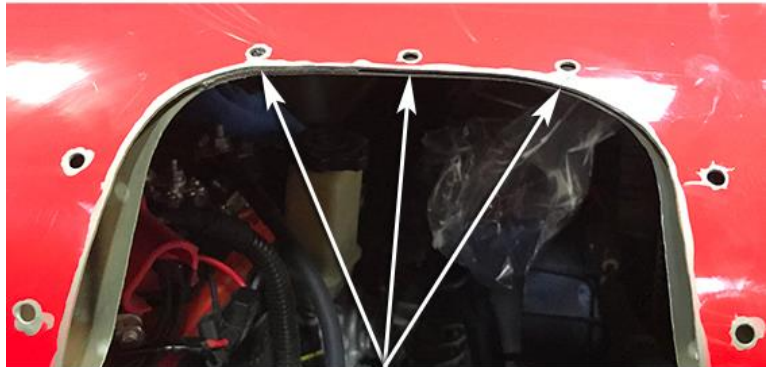
Install M5 Body Washer(s) - (if no seam sealer)
