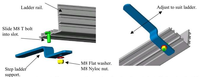
The Stepladder support can be positioned on the rail to suit the ladder length and width being carried.
