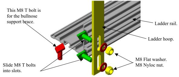
The Ladder hoop can be adjusted on the rail to suit the ladder length and width being carried.
