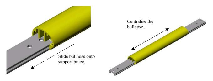
Assemble the bullnose support brace onto the underside of the ladder rails using the M8 T bolts located into the T slot prior to fitting the rear bullnoses. Assemble the M8 flat washers and M8 nyloc nuts, do not fully tighten the nuts as some adjustments may be required when fitting the ladder rails to the crossbars.
