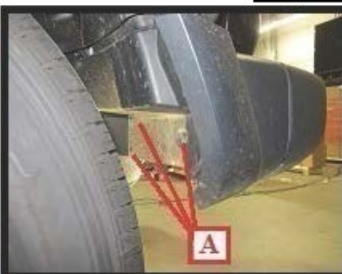
Remove passenger and driver side splash guards by removing 3 screws (A) shown above with an 8mm socket
