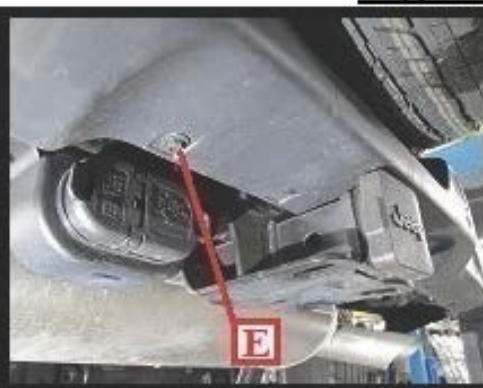
Remove screw (E) above both driver and passenger sides using a 10mm socket drive
