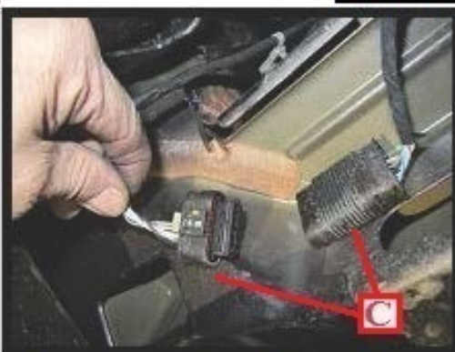
Pull out on white tab (D) in the direction of the red arrow shown in Fig. 46 to release connection lock then pull apart sensor connection (C) as shown in Fig. 47
