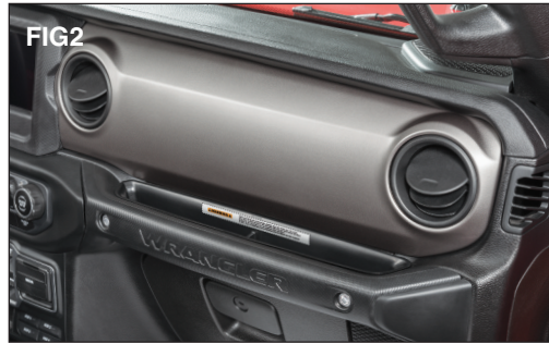
All Jeep model-year versions of the Grab Handle Storage Tray should sit flush behind grab bar as shown. (FIG 2)
