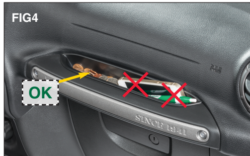
The photos above illustrate the INCORRECT way to fill the tray with objects. Any item that sticks out of the tray could contact occupants in the event of an SRS Airbag deployment.
