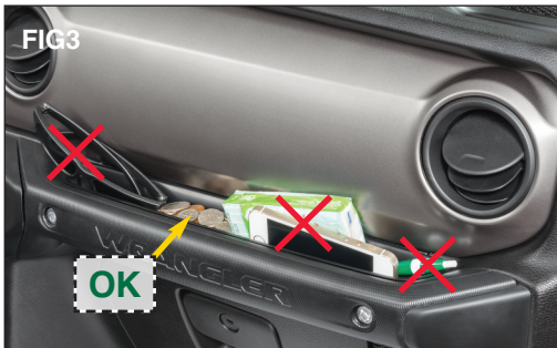
Any and all objects you place in the storage tray must not exceed the depth of the storage tray. Pens, coins and small objects that fit below the top surface of the grab bar are acceptable.
