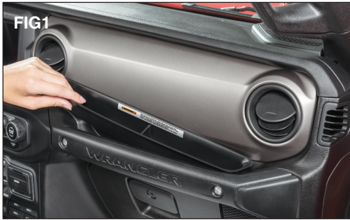
Put on safety glasses. Drop in and press down to snap your Grab Handle Storage Tray into position. (FIG 1)
