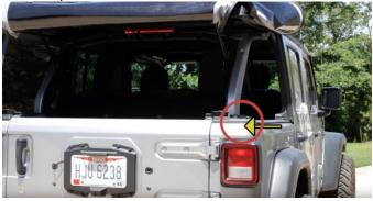
With a flat head screw driver, remove the tail light bolt cover, located just above each tail light in the interior panel.
