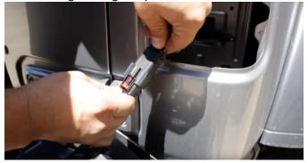
Resecure the tail light retaining bolt with a T40 Torx bit.
