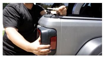
Disconnect the light from power by pulling down on the red tab, pinching the white tab, and pulling away.
