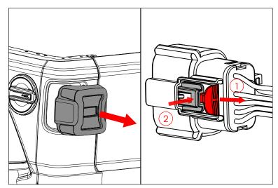
3. Remove OE Mounting Bracket by unscrewing Phillips Head Screws. Disconnect Electrical Plug on the back of LED Tail Light.
