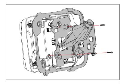
5. Reattach Electrical Plug from Step 3 to LED Tail Light. Using supplied Bolts, attach Guard to Rear Housing.
