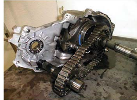
(Fig. 11) Front Drive Chain & Shaft Removal
