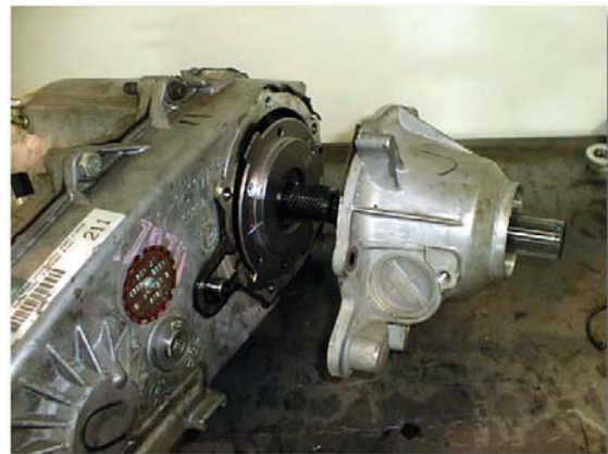
(Fig. 8) Rear Tailhousing Removal
