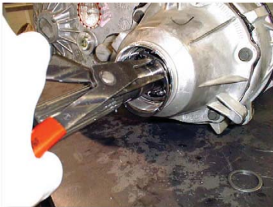
(Fig. 6) Rear O.D. Snap Ring Removal
