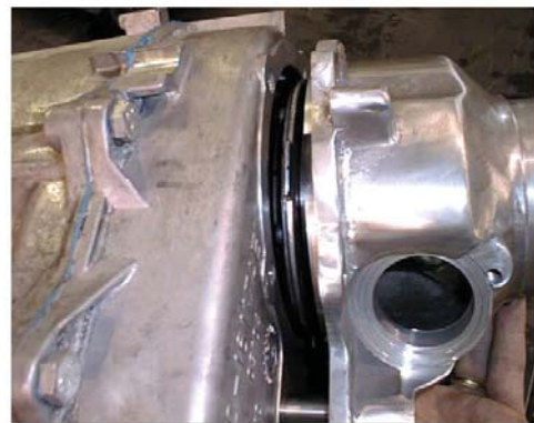
(Fig. 12A) Tailhousing Installation
