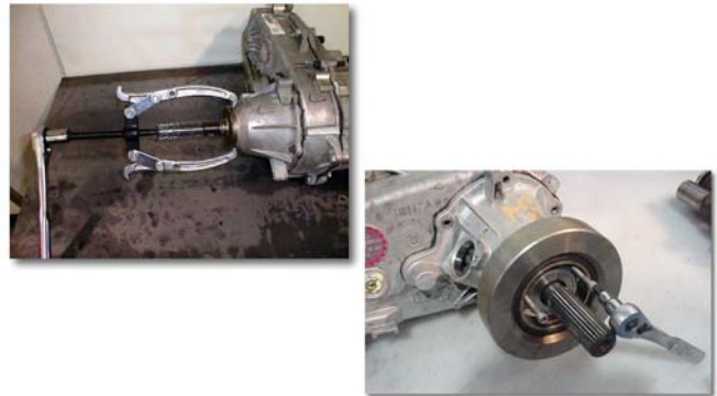
(Fig. 3) Slinger Removed / Harmonic Dampener
