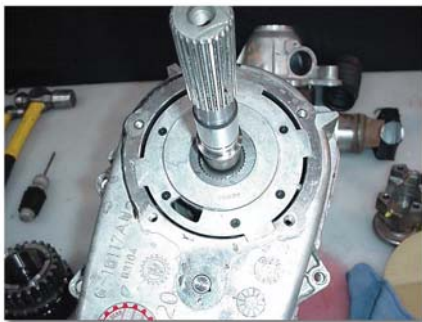
(Fig. 10) Oil Pump Removal
