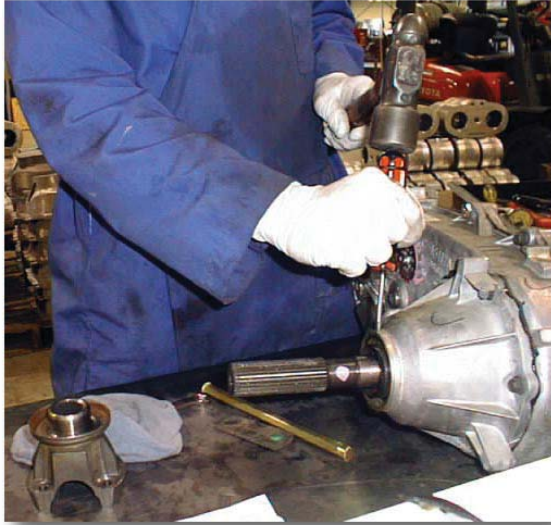
(Fig. 5) Rear Seal Removal
