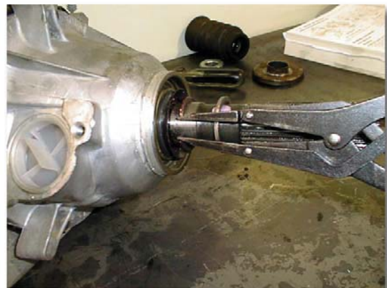
(Fig. 4) Stop Spacer & Snap Ring Removal
