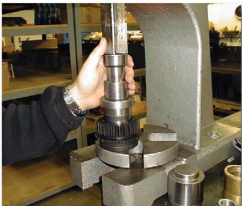
(Fig. 2A) Pull the Needle Bearings Out
