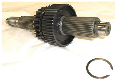
(Fig. 4A) (Large) Retaining Ring Installation
