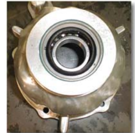
(Fig. 11A) Seal Installed
