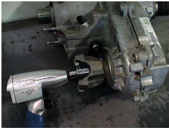
(Fig. 1) Yoke Nut Removal
