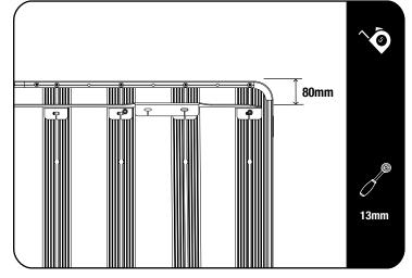
After fitting the wind deflectors, the tray should still be upside down, loosely mount the Foot Rails (Item 17L & 17R from FAJK008 box) to the Tray using M8 x 16 Hex Bolts, M8 X 16 X 1.6SS Flat Wahsers and M8 Nyloc Nuts (Items 16, 18 & 19). As before use the machined slots to insert the hex bolts into the Slats. The Foot Rail should be mounted at the opposite end of the Tray to the wind deflector.
