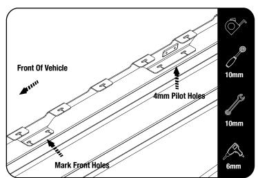
Align the Foot Rail with the rib on the roof so that it runs parallel with the rib before marking the two front holes.
