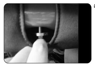
Pull back the padding around the roll bar above the rear seats and insert an M8 x 75 Hex Bolt and M8 Large Washer (Items 14 & 15 from FAJK007 box) through the hole as shown.
