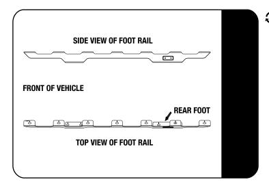
Place the Foot Rail on the roof and align the rear slots of the Foot Rail centre with the holes drilled in 2.3.
