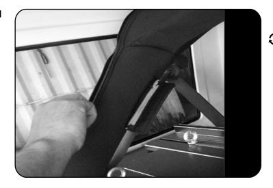
Loosen the velcro, unzip and remove the padding covering the roll bars.
