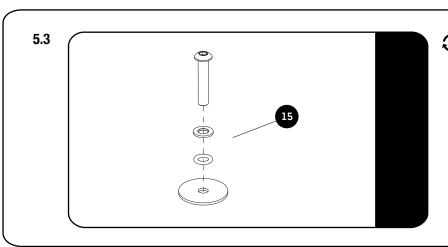
Should you wish to remove your rack, you will need to plug the holes you drilled in the roof (Step 3.4), using the supplied Sealing Plug Assemblies.
