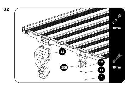
The Foot Rail should still be loose enough to move. Line the brackets up with the holes on the roof and fasten them into position using M6 x 30 Hex Bolts, M6 x 19 x 1SS Flat Washers, M6 x 12 x 1SS Flat Washers and M6 Nyloc Nuts (Items 6, 7, 11 & 12). Centre the tray from left to right. Use a tape measure to double check. Once you are happy that the Tray is in the correct position, fasten all the nuts and bolts, both inside and outside of the vehicle on all brackets that were installed.
