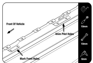
Align the Foot Rail with the rib on the roof so that it runs parallel with the rib before marking the two front holes.
