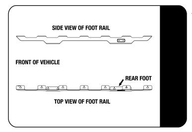
Place the Foot Rail on the roof and align the rear slots of the Foot Rail centre with the holes drilled in 2.3.
