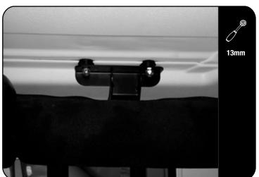
From the inside of the vehicle, in the same position as where you just inserted the bolt in 3.4, push the Middle Support Bracket (Item 2LH & 2RH) through the hole in the roll bar padding and loosely fasten it to the roll bar.
