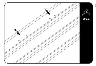
Change the 4mm drill bit to a 22mm hole saw. From the outside of the vehicle, drill all the 4mm holes (8 in total) out to 22mm.
