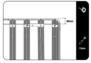
After fitting the wind deflectors, the tray should still be upside down, loosely mount the Foot Rails (Item 17L & 17R from FAJK008 box) to the Tray using M8 x 16 Hex Bolts, M8 X 16 X 1.6SS Flat Wahsers and M8 Nyloc Nuts (Items 16, 18 & 19). As before use the machined slots to insert the hex bolts into the Slats. The Foot Rail should be mounted at the opposite end of the Tray to the wind deflector.
