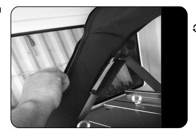
Loosen the velcro, unzip and remove the padding covering the roll bars.
