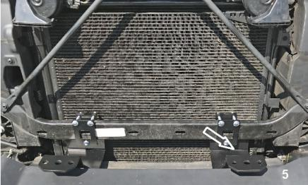
5. Pay attention to picture #5, take notice of the off set in the brackets. Lay the brackets out to match picture #5. (Bracket Alignment and Off Set shown in picture #5 is the position needed to install the Quadratec LED Light Bar,
