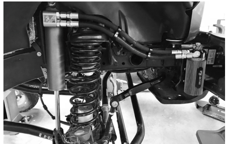
Figure 15: Final installed shock. Passenger side shown
