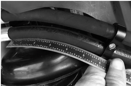
Figure 13: Clamp 1. Passenger side shown
