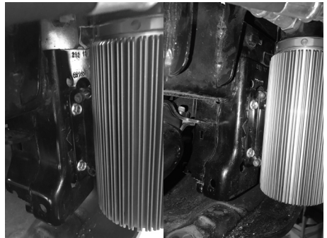
Figure 12: Loosely install 1/4-20 hardware. Passenger side shown
