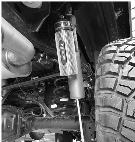
Figure 15: Final installed shock. Passenger side shown
