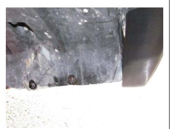
110. Mark and drill two Ø7mm holes through each of the inner guards in line with the cage nuts.
