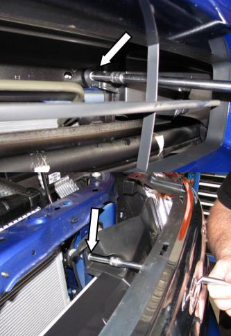
7. Using a socket extension, remove the screws holding the inner grille air deflectors to the vehicle. Place in a safe place.
