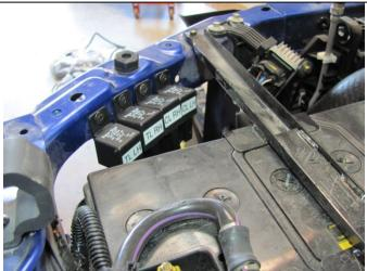
29. Using the tek-screws provided, attach the 3 relays to the panel directly behind the LH head light as shown.
