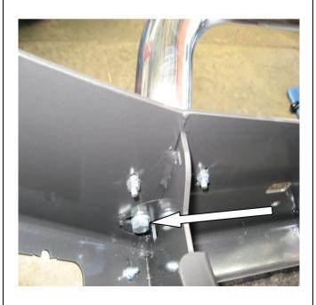
90. If fitting Top Tube, fasten with two M12 x 40 Bolts, spring and Flat Washers.
