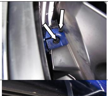
Undo and remove the screws and plastic clips behind the grille near the lower inner edge of the head lights.
