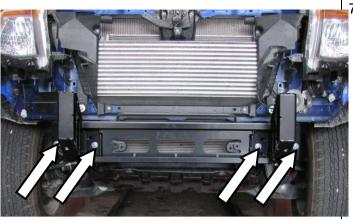
75. Attach the mount bracket to the chassis end plates using four M10 SEMS bolts into the captive nuts. Leave loose at this stage.
