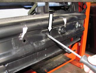
Use a screw driver to push the two plastic clips inward from the front cross beam.
