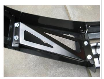
101. Fasten the (L&R) Wing Braces using M10 SEMS bolts and Flange nuts (four each per side)
