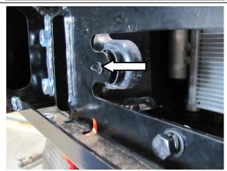
84. Using the original plastic clips re-fit the factory air deflector to the two holes in the mount bracket.
