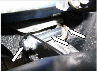
82. Secure the rear of the chassis braces to the chassis using two M10 x 80 bolts, two M10 spring washers and two M10 flat washers through two crush tubes into the nut plate assemblies on each side of the vehicle. Leave loose at this stage.
