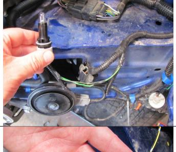
32. On the left side of the vehicle, carefully cut back the protective tubing from the clearance light globes wiring being careful not to damage the wires inside.
