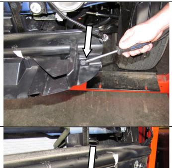
9. Remove the plastic panel attached to the front cross beam by removing the plastic clips. Discard the panel.
