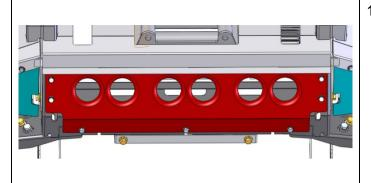
112. Attach the centre stone shield to the mount bracket using seven M8 hex bolts, seven M8 spring washers and seven M8 flat washers into the cage nuts fitted in step 80.
