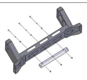
81. Attach the OE stone shield bracket to the chassis mount using three M8 x 25 black bolts, three M8 black flat washers, three M8 black spring washers and three M8 flange nuts. Leave loose at this stage.
