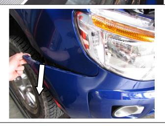
8. Starting on the RH side of the vehicle, carefully pull the rear most corner away from the vehicle un-clipping the bumper. With the assistance of another person remove the bumper from the vehicle and place in a safe place where it will not be damaged. Disconnect the sensor attached to the bumper and allow it to hang loose. If fog lights are fitted they will need to be disconnected.
