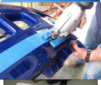
49. Using a jig saw or similar, carefully cut along the line made in the previous step.
