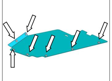
105. Fit four M6 cage nuts to each of the under wing panels as shown.
