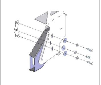
93. Attach the bar to the mount bracket using six M12 bolts, six M12 spring washers and six large diameter M12 flat washers, into the nut plates which are placed inside the box upright sections of the mount bracket. Leave loose at this stage.
