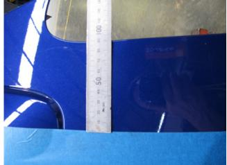
Note: The line should end up being 90mm below the edge of the bumper that mates with the vehicles guard.
