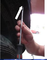
4. Remove all the bumper fasteners along the inside edge of the wheel arches.
