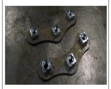
91. Fit three M12 cage nuts to each of the cage nut plates as shown.
