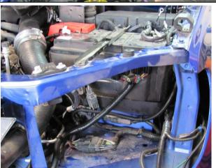
Route the battery positive and the battery negative wires to the relevant sides of the vehicles battery. Do not attach at this stage.
