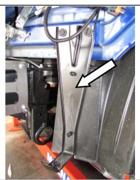
Remove and discard the inner guard support brackets from both sides of the vehicle.
