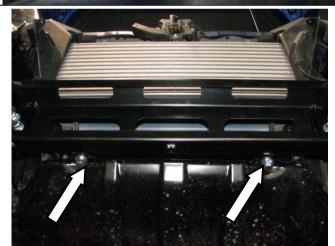
83. Re fit the OE stone shield to the bracket fitted in step 81 using two M10 SEMS bolts and two M10 flange nuts.
