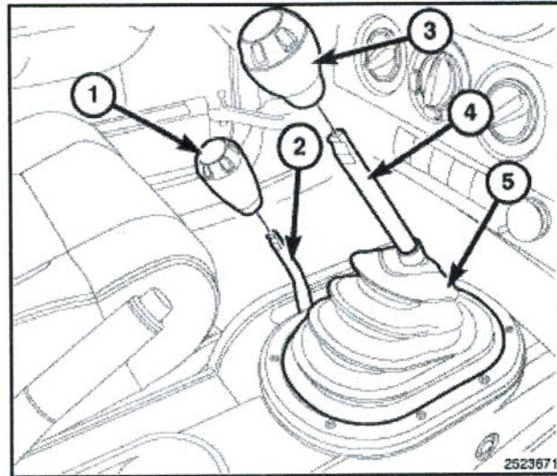
2. If removal of the shift knob (3) by hand is not possible wrap a shop towel (4) or equivalent around the base of the shift knob (3) and using puller C-4333A-1 or equivalent (2) and slide hammer (1), remove the shift knob (3) from the shift lever.
